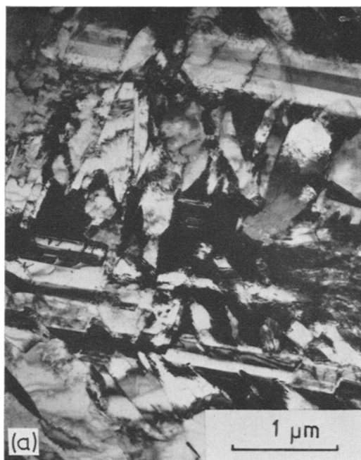
Figure 5 Alloy A Fe-16 wt % Cr-12 wt % Ni. Structures after heating partially martensitic specimens for 2 min (a) at 550°C (b) at 575°C, showing stacking faults and twins within the reversed \gamma regions.
